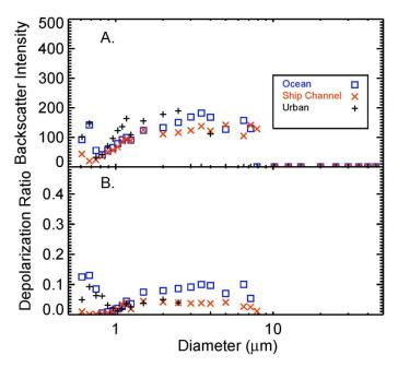
As can be seen, the transported aerosol population (Ocean) contained particles with much higher depolarization rations than either the Urban or Ship Channel
